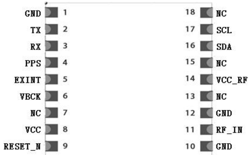
Figure 2: Pin Assignment
